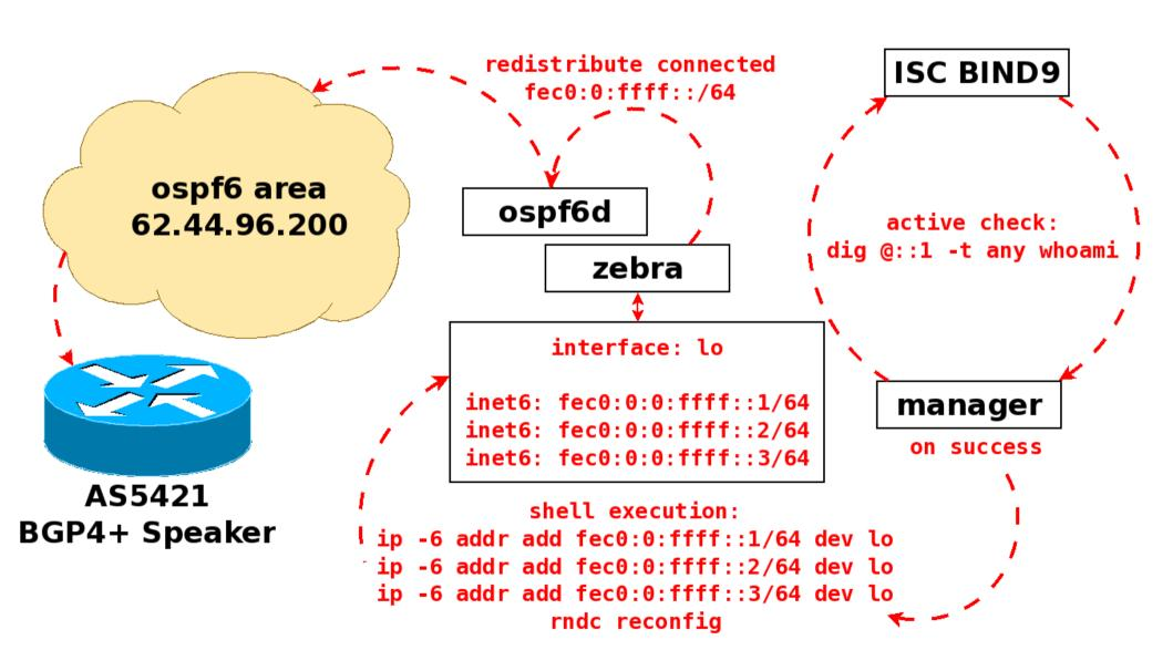
How does DNS anycast node work: stopping the prefix redistribution on BIND9 failure
